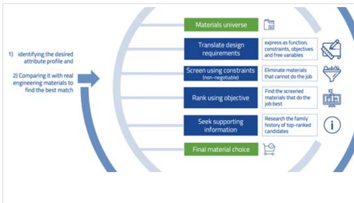
Figure 1: Materials selection procedure by Ashby, et al. [1].
